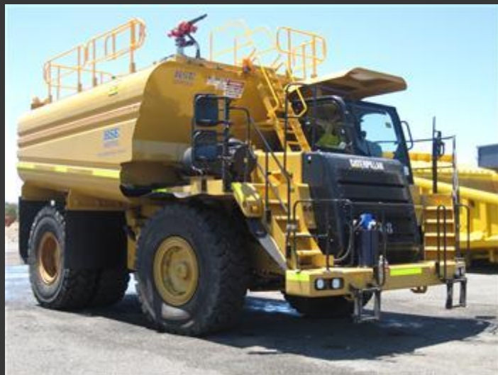
CAT777F water cart
